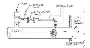
Chlorination of a pipeline is conducted using gaseous chlorine dissolved into a carry water stream of 50 gpm
