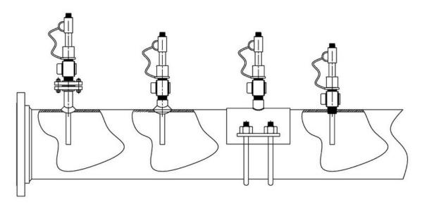
Flanged Installation Drill & Tap blind flange for Retractable Injector. Maximum versatility.
