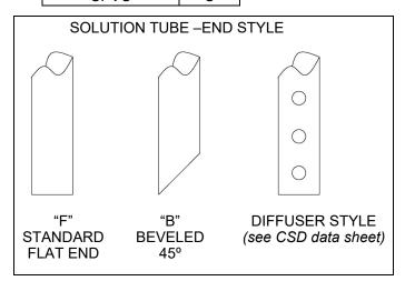
SOLUTION TUBE -END STYLE STANDARD FLAT STYLE AND BEVELED END STYLE ARE SHOWN ON THIS DATA SHEET.
